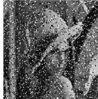
Figure 6.2 (b) Received image (2x1) (SNR=1 dB, PSNR=14.9546dB)
