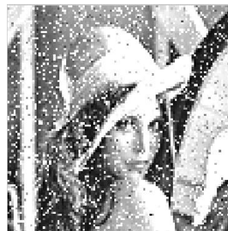
Figure 6.9 (b) Received images (2x2) (SNR=14 dB, PSNR=18.7313 dB)
