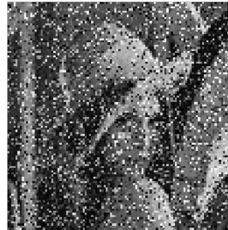
Figure 6.1 (b) Received image (1x1) (SNR=1 dB, PSNR=13.8877 dB)
