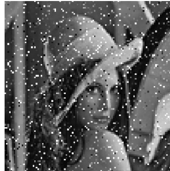
Figure 6.7 (b) Received images (1x1) (SNR=15 dB, PSNR=17.4777 dB)
