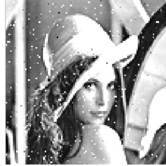
Figure 6.3 (f) Received images (2x2) (SNR=7 dB, PSNR=26.2210dB)
