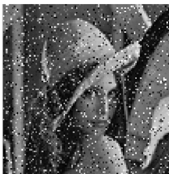
Figure 6.8 (c) Received images (2x1) (SNR=15 dB, PSNR=18.9848 dB)
