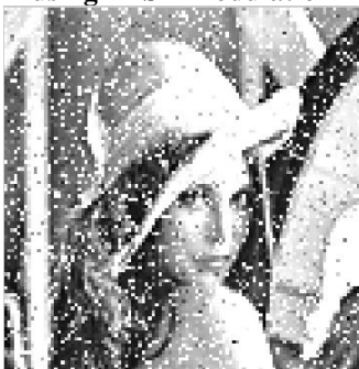
Figure 6.3 (c) Received images (2x2) (SNR=3 dB, PSNR=19.1228dB)
