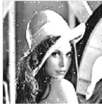
Figure 6.9 (e) Received images (2x2) (SNR=19 dB, PSNR=27.8024 dB)
