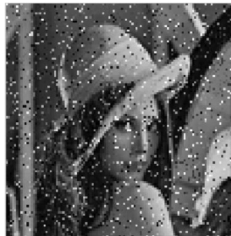
Figure 6.1 (g) Received image (1x1) (SNR=8 dB, PSNR=19.3317dB)
