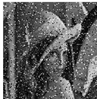
Figure 6.1 (d) Received image (1x1) (SNR=5 dB, PSNR=14.9546dB)
