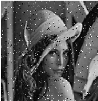
Figure 6.2 (e) Received image (2x1) (SNR=6dB, PSNR=20.9395dB)
