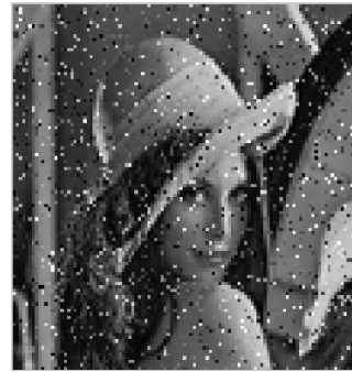
Figure 6.1 (f) Received image (1x1) (SNR=7 dB, PSNR=18.2804dB)
