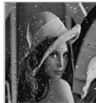
Figure 6.2 (h) Received images (2x1) (SNR=9dB, PSNR=25.4945dB)
