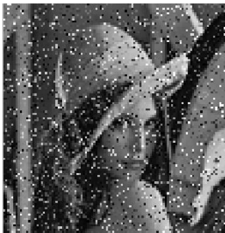
Figure 6.2 (c) Received image (2x1) (SNR=3 dB, PSNR=17.2246dB)
