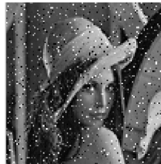
Figure 6.2 (d) Received images (2x1) (SNR=5 dB, PSNR=19.6950dB)
