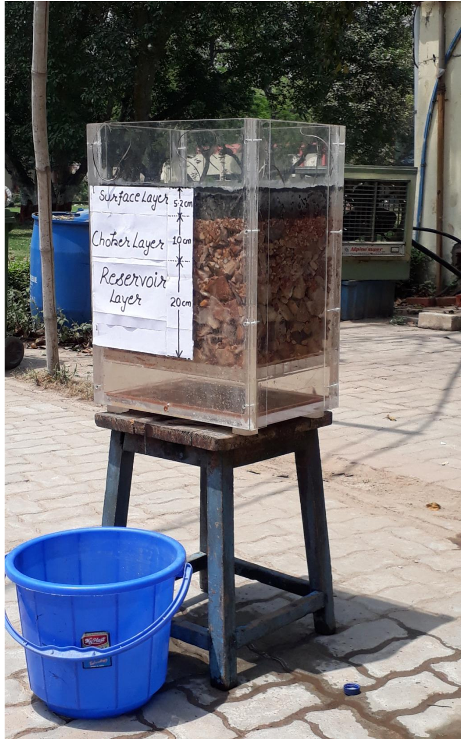
Figure 4. 10 : Prototype Showing Layers in Porous Asphalt Pavement
