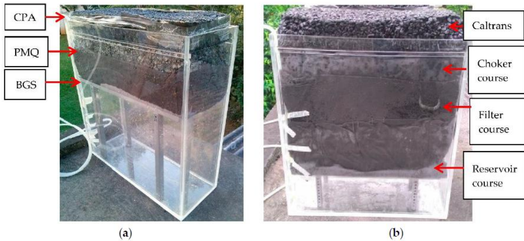
Figure 2. 5 : Two Model (a) and (b) Consisting of Three and Four Layers of Porous Asphalt Pavement
