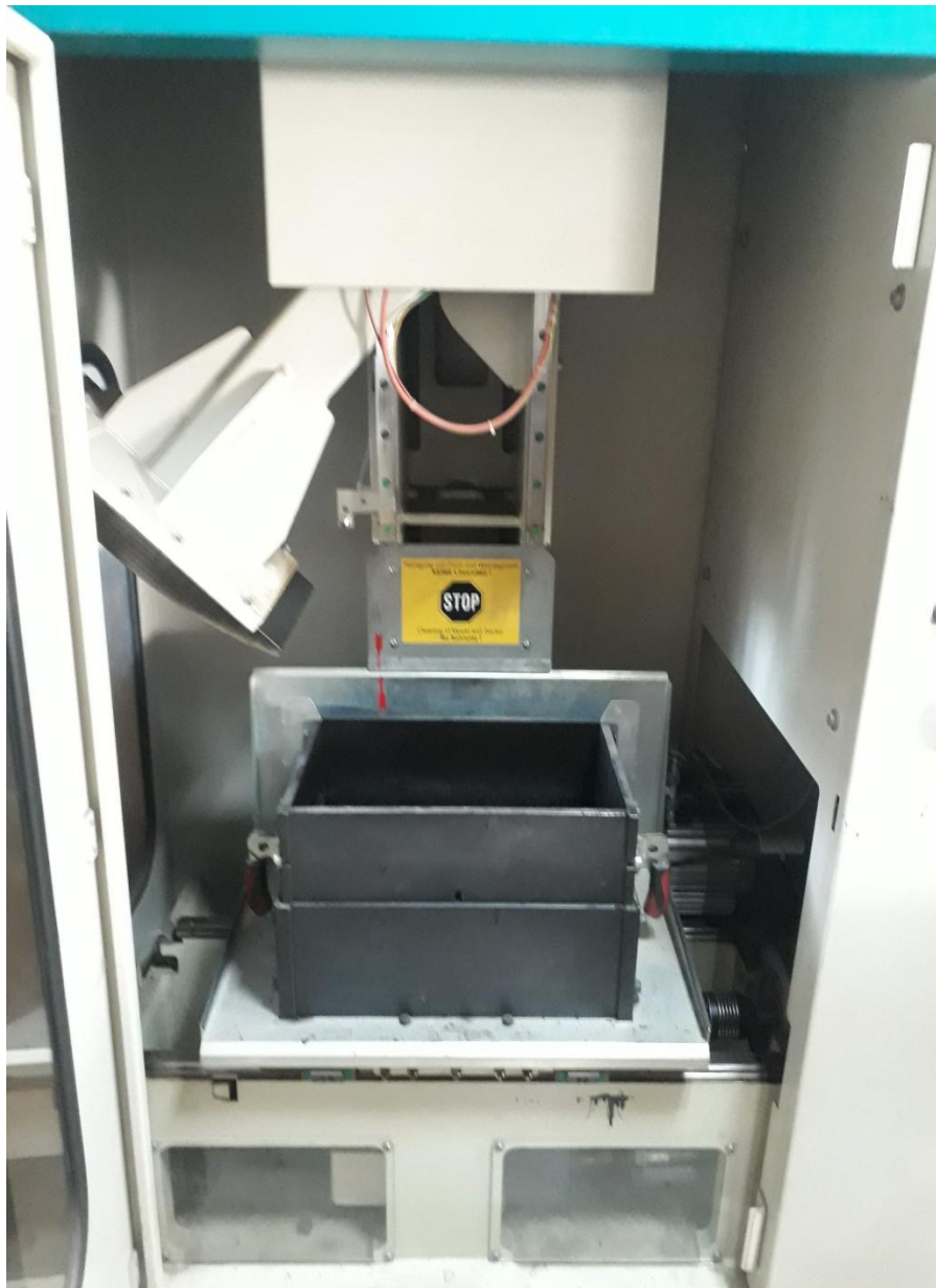
Figure 3. 25 : Inside View of Slab Casting Machine
