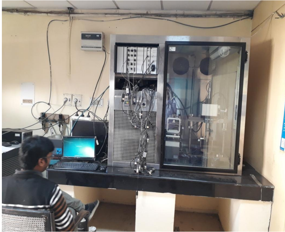
Figure 3. 23 : Complete Setup of Dynamic Creep Test
