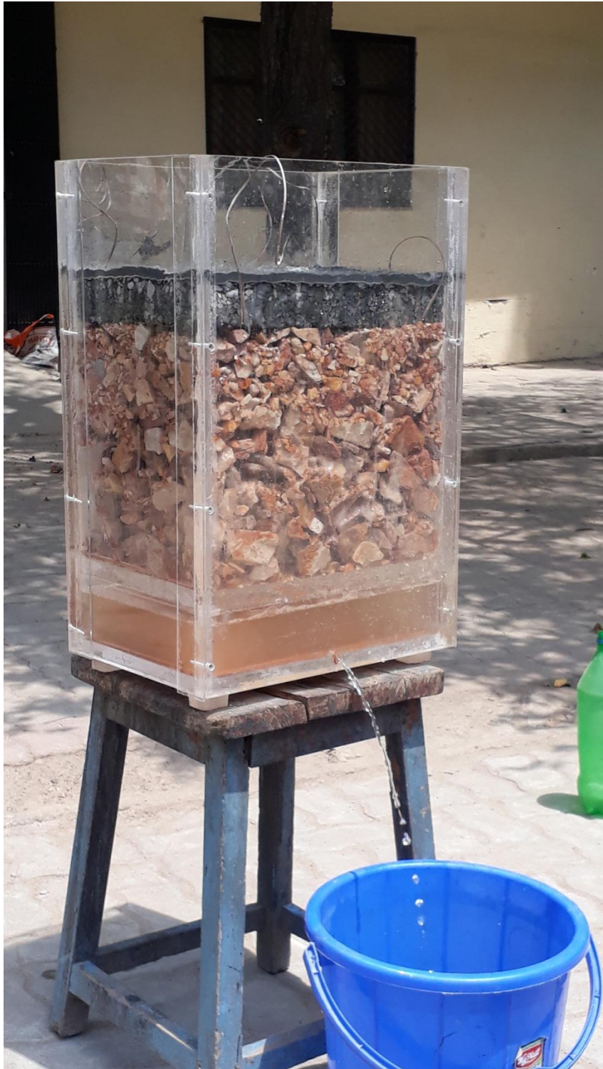
Figure 4. 9 : Prototype for Porous Asphalt Pavement
