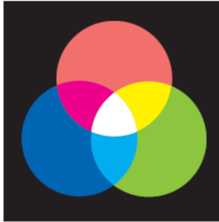
Fig 3.2: Projections of three lamps with the colors red, green and blue onto a wall in a dark room
