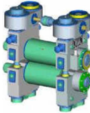
Figure 1.2 Housing of Rolling Mill
