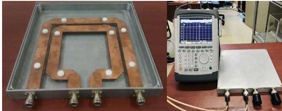
Figure 3.30: Photograph of fabricated directional coupler.
