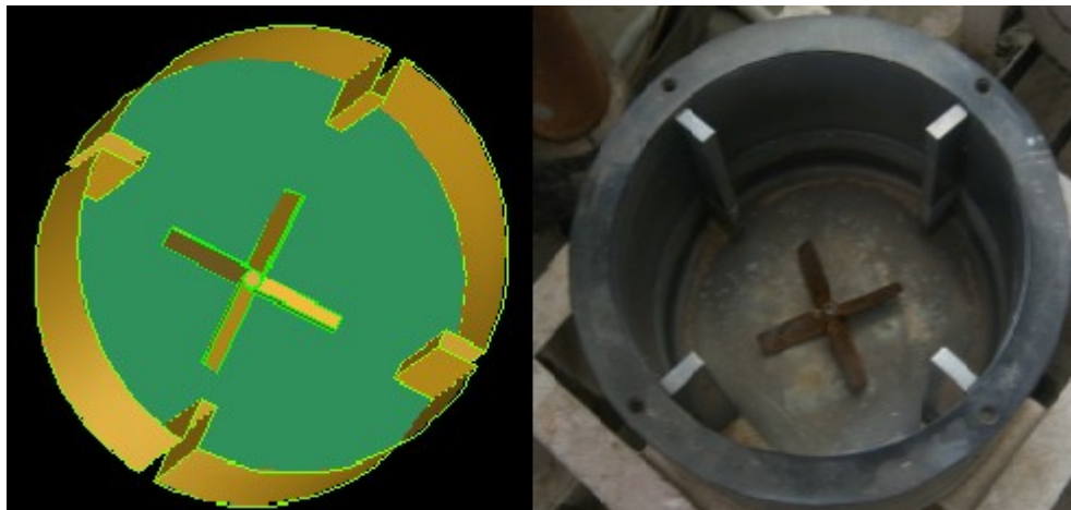
Figure 5.3: a) CAD model of fluid volume with propeller b) Cylinder with propeller
