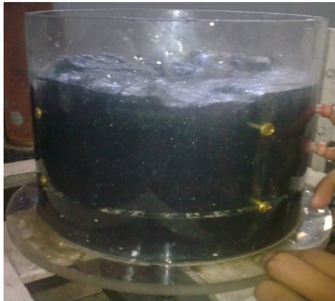
Figure 4.3: Aluminium tank replaced by a transparent tank of equal size
