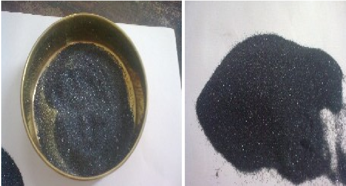
Figure 4.7: Silicon carbide particles retained between 500-600 micron size sieves
