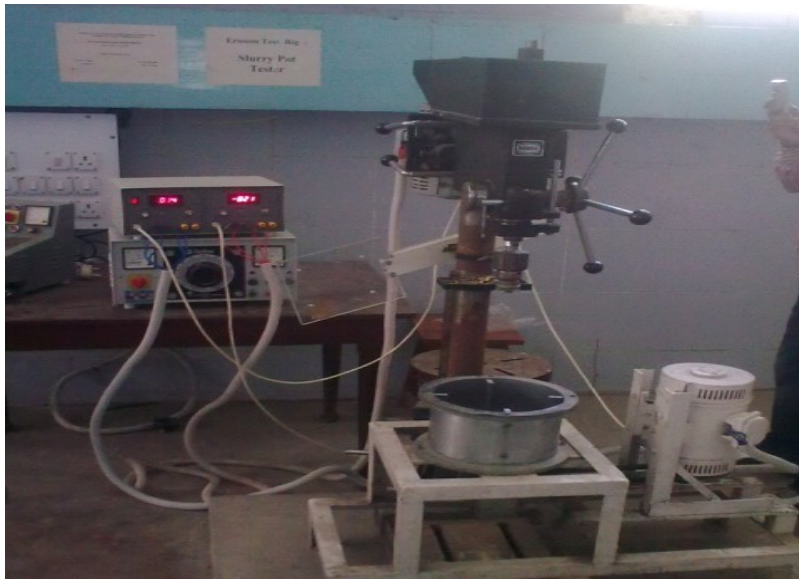
Figure 4.2: Slurry pot tester with speed control unit
