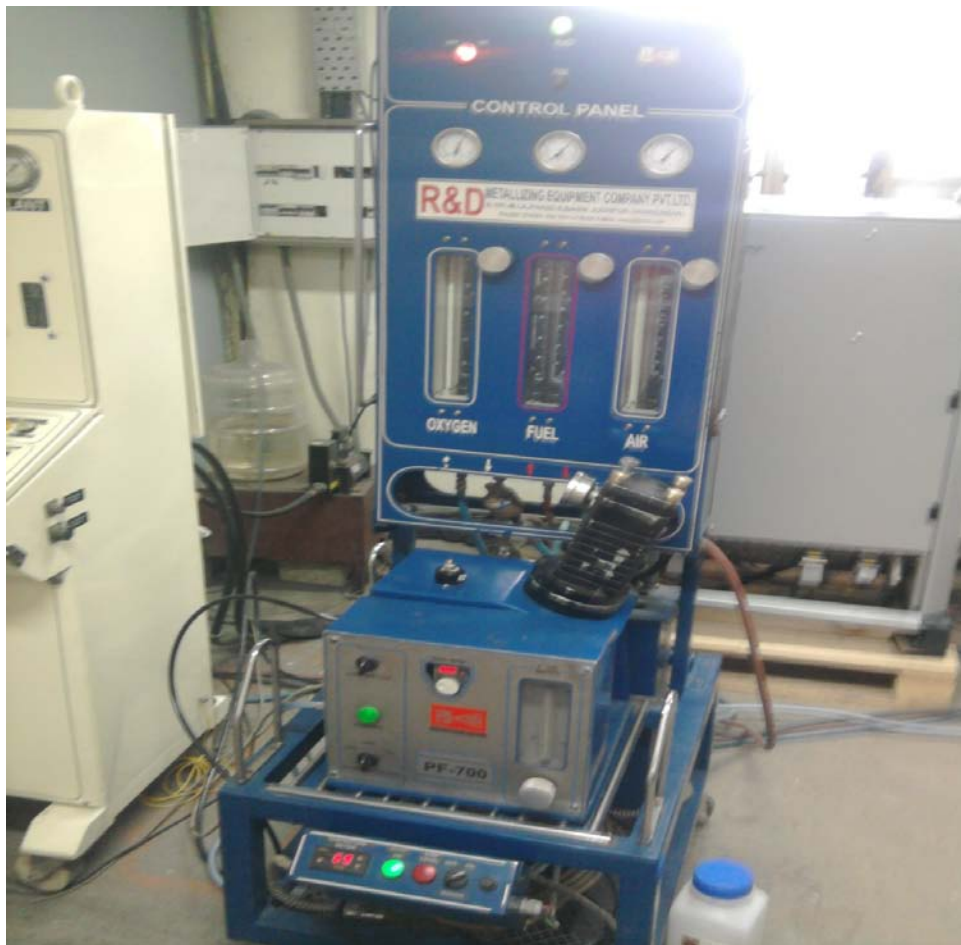
Figure 5.4 High Velocity Oxy-Fuel (HVOF) Coating Machine.
