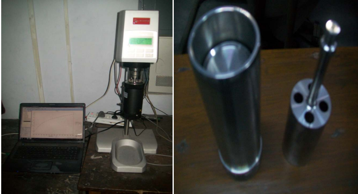
Figure 3.6 (a) Rheometer (Anton Paar) Figure 3.6 (b) Cylindrical cup and rotating Bob
