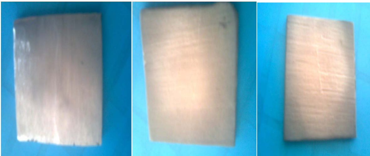
(a) Uncoated 13Cr4Ni Steel
