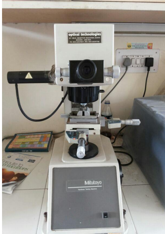
Figure-3.1 Vicker's Microhardness
