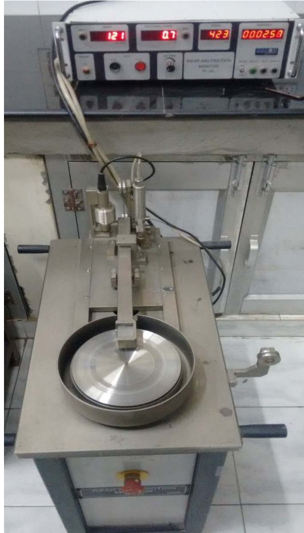
Figure 3.3: Images of pin on disc setup for wear test (Ducom-TR-20CH-400).
