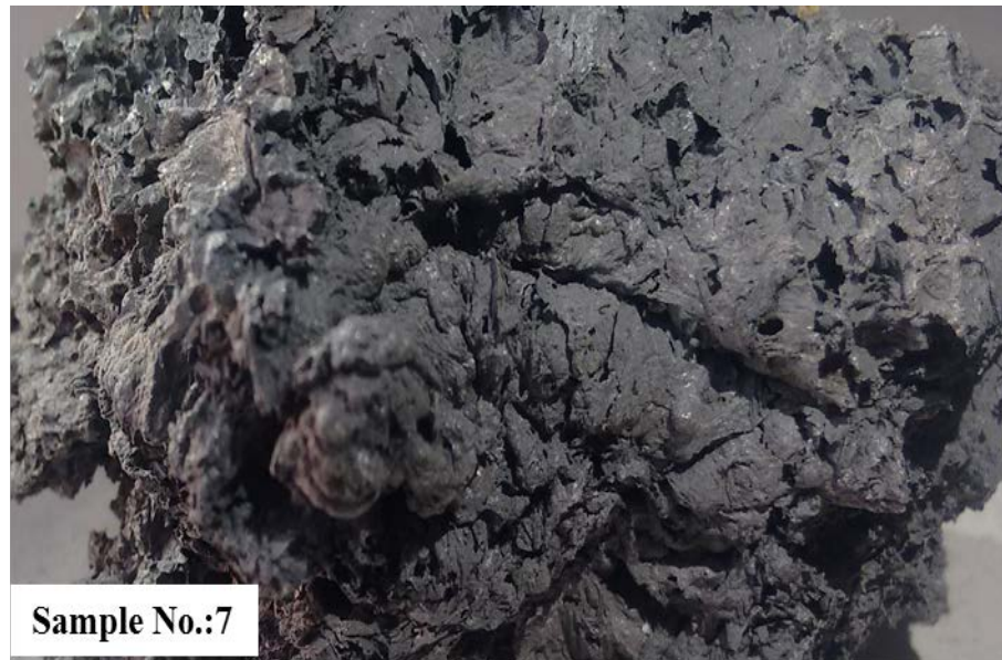
Figure 5.7: Photograph of sample AMCF- ^{10}F_{\text{fine-0.70}} collected after blast test.
