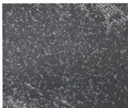
Figure 3.74 Photomicrograph of Ti 31 (100x) [Exp. No.2]
