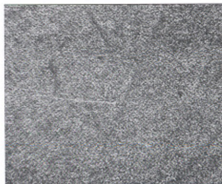
Figure 3.98 Photomicrograph of Ti 31 (100x) [Exp. No.14]
