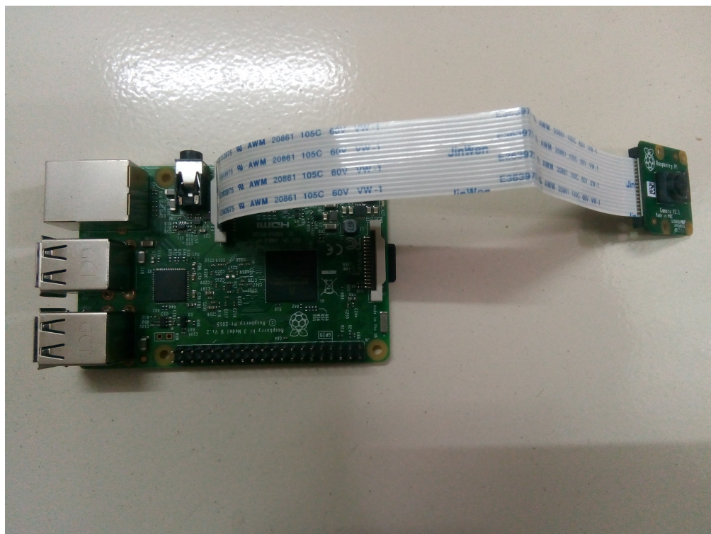
Figure 4.14: Raspberry Pi attached with its camera module
