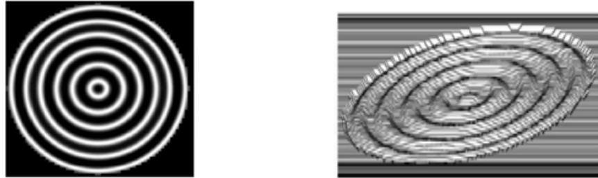
Fig.1.24: Surface error caused by uneven cooling of the machine or the part during fabrication; (Richard et al. 2003)
