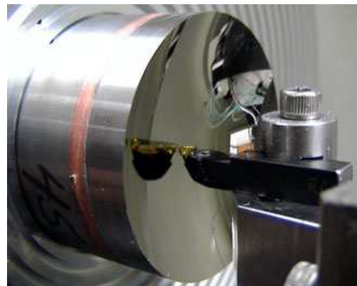
Fig.1.21: Changing of cutting point along tool edge; (Richard et al. 2003)
