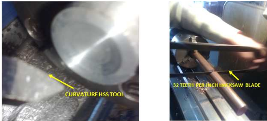
Fig.3.15: Blank prepared on the conventional lathe machine
