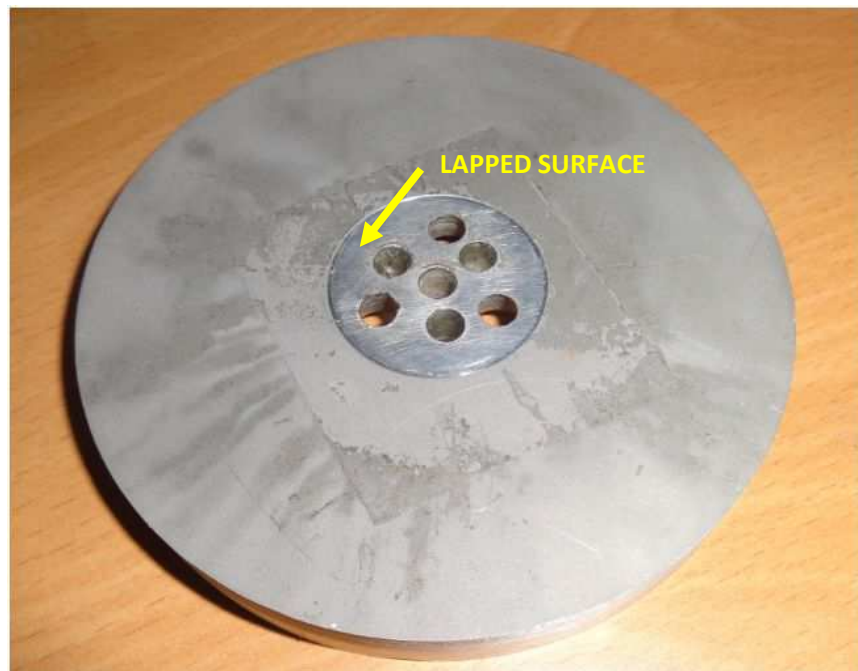
Fig.3.17: Lapping of the Al6061 fixture
