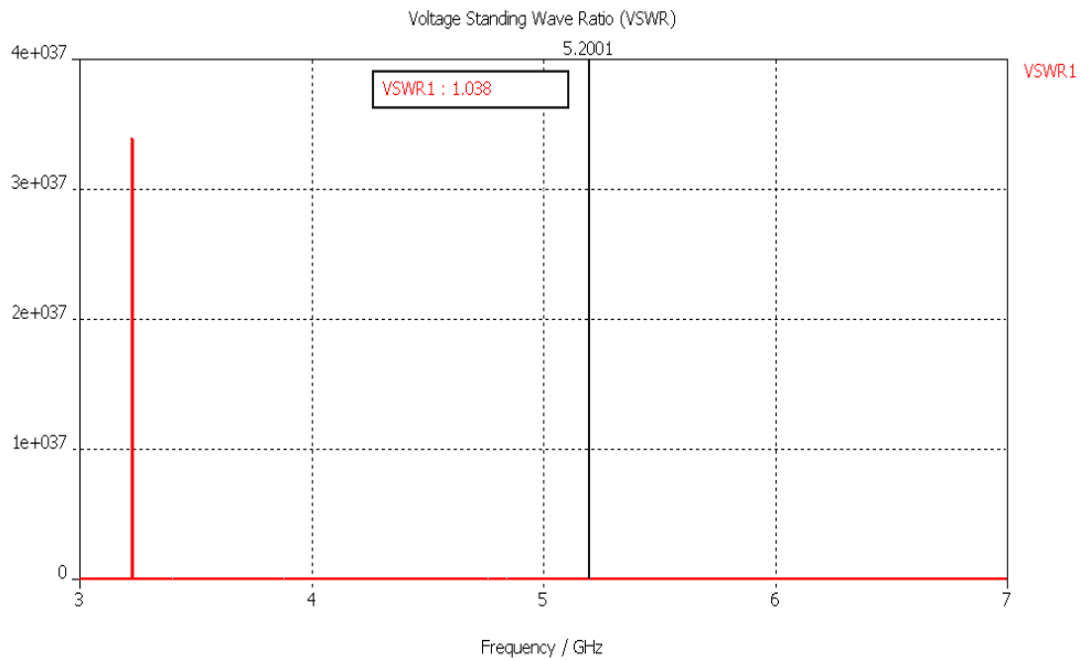
Figure 4.6 VSWR Versus Frequency Plot of coaxial feed antenna
