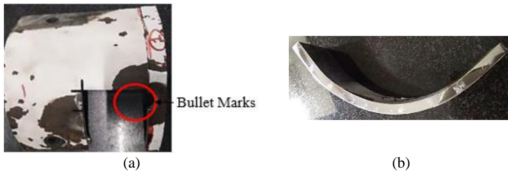
Fig.5.5 (a) Test specimen of bullet penetrated bend plate and (b) Hardness measurement points on bullet penetrated bend plate
