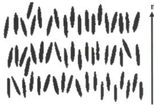
Fig. 1.8 Molecular arrangement in a SmA phase. The long axes of the molecules in each layer, on an average, are perpendicular to the layer plane containing the molecules
