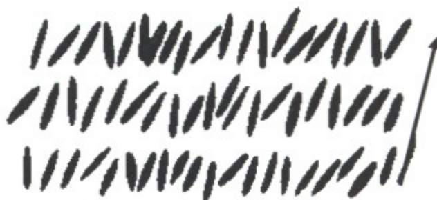
Fig. 1.10 Molecular arrangement in SmC phase. Molecular tilt at an angle with respect to layer normal is seen
