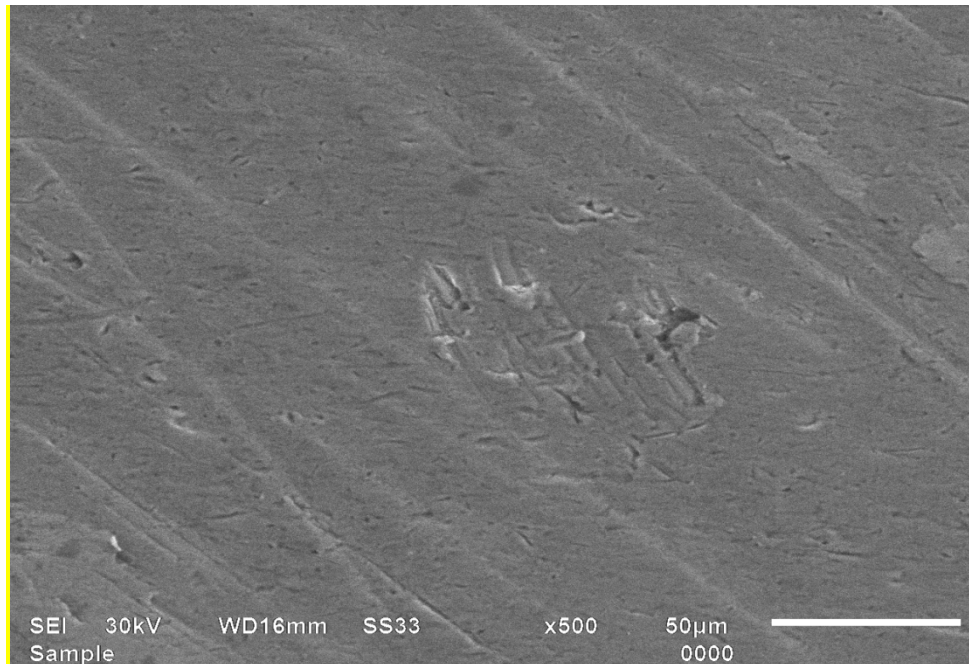
Figure 4.10 SEM of uncoated steel 316 before wear
