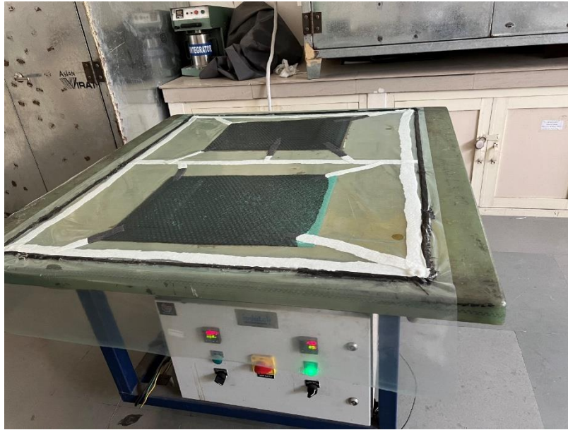
Figure 3.11: Preparation of nano reinforced fiber sheets on VARIM
