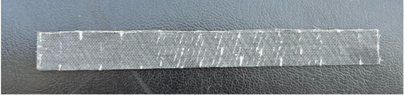
Figure 3.17: Sample for flexural testing
