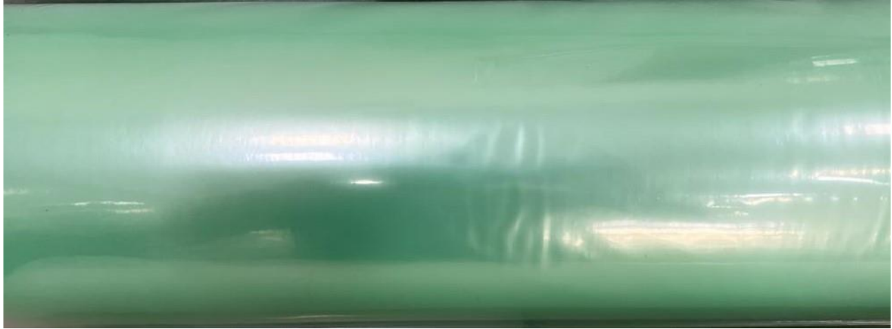
Figure 3.7: Laminating sheet used for covering the mold surface
