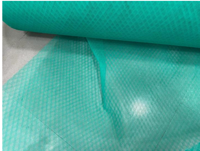
Figure 3.4: Infusion mesh for covering the sheet
