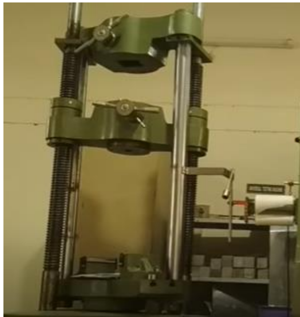
Figure 3.15: Universal Testing machine for tensile testing (PU, Chandigarh)
