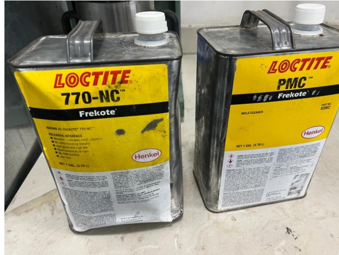
Figure 3.5: Mold Cleanser and Releasing agent for the mold surface
