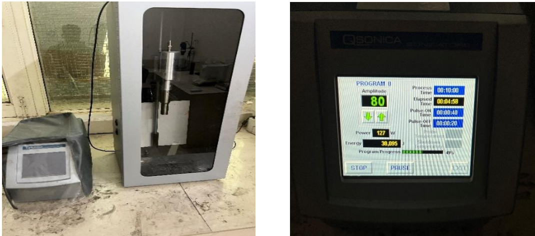
Figure 3.9: (a) Probe Sonicator machine (b) Digital display for the procedure
