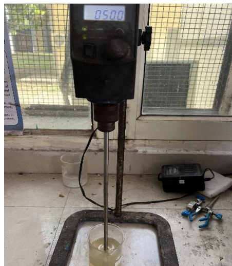
Figure 3.10: Mechanical stirrer for mixing the hardener
