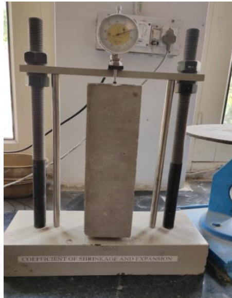
Fig 3.21: Testing setup for drying shrinkage
