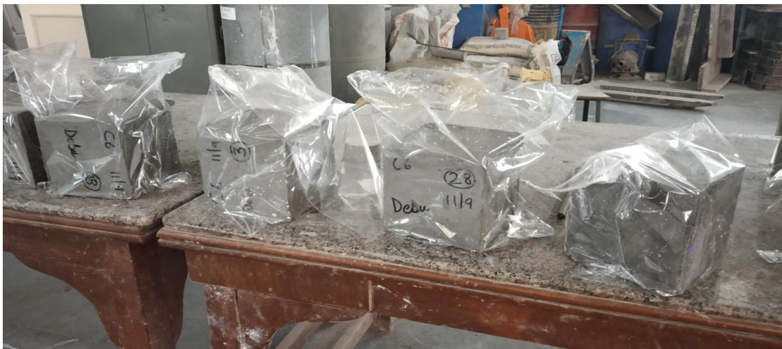
Fig. 3.14: Specimens sealed in plastic bags for post conditioning
