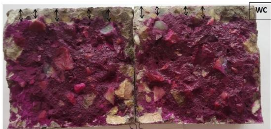
Fig. 3.28: Measurement of uncoloured part after Phenolphthalein spray
