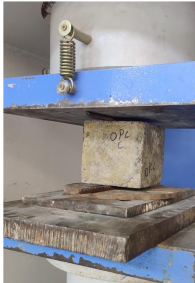
Fig. 3.27: Test setup for splitting the cube specimens
