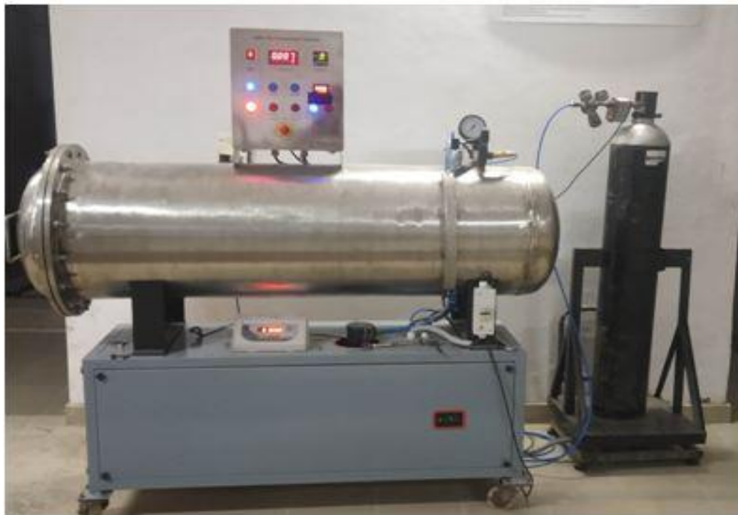
Fig. 3.10: Accelerated carbonation curing chamber used in the present study
