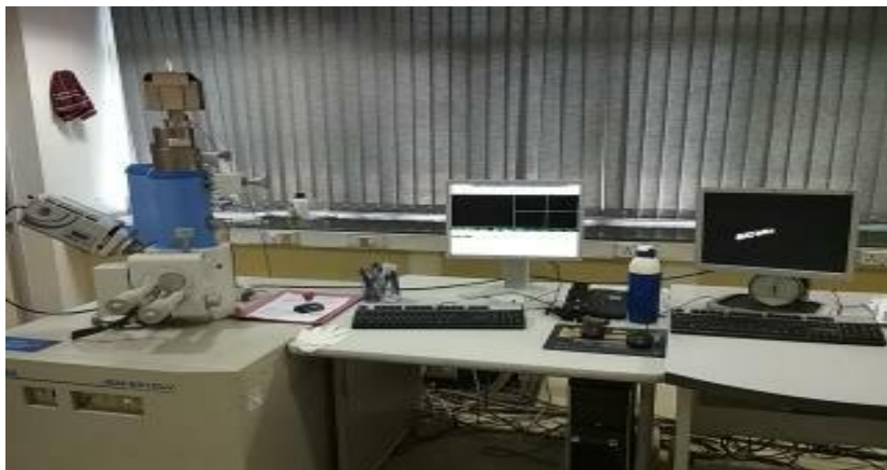
Fig. 3.24: Experimental set up for SEM and EDS spectroscopy
