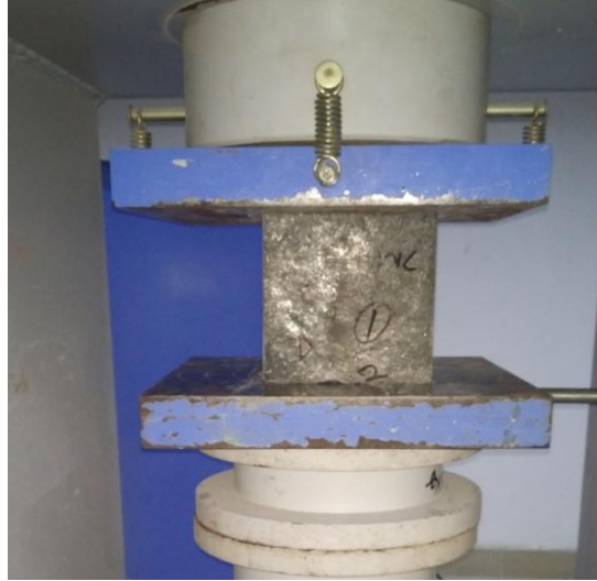
Fig. 3.15: Compressive strength test of concrete
