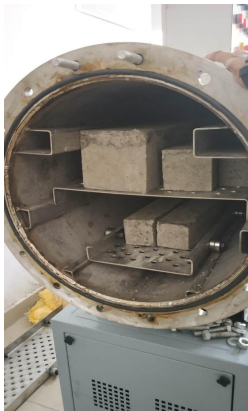
Fig. 3.13: Specimens placed in carbonation chamber
