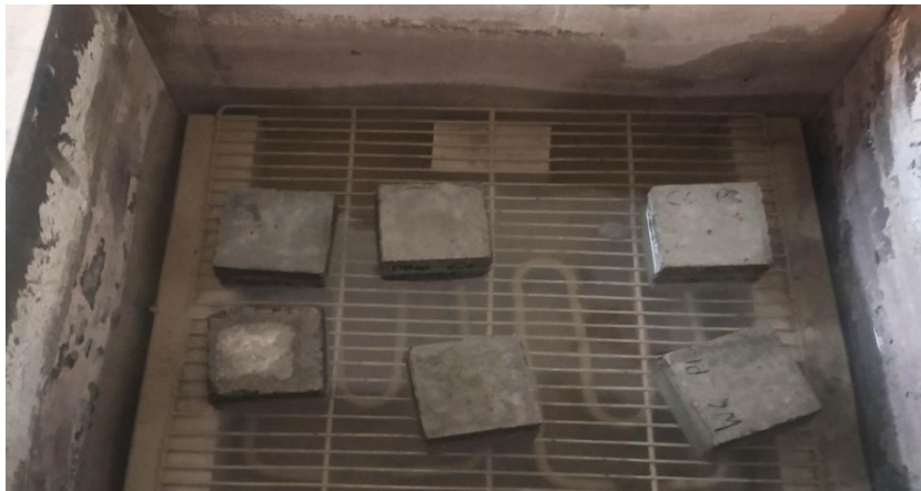
Fig. 3.8: Temperature controlled water curing of concrete
