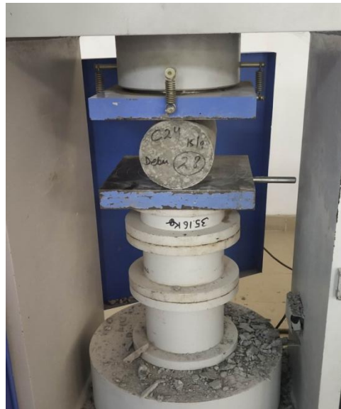
Fig 3.16: Test setup for Split Tensile Strength
