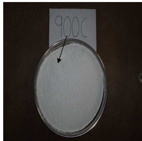
Fig.4.6 Eggshells powder at 900°C
