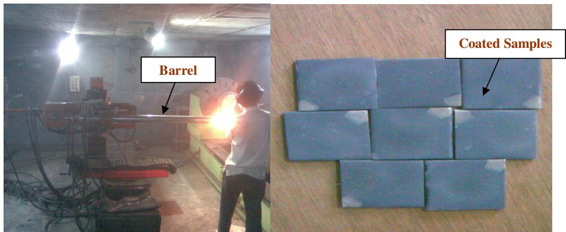
Fig.4.45 Performing coating process
