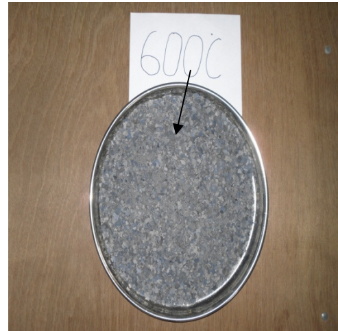
Fig.4.8 Eggshells powder at 600 0 C
