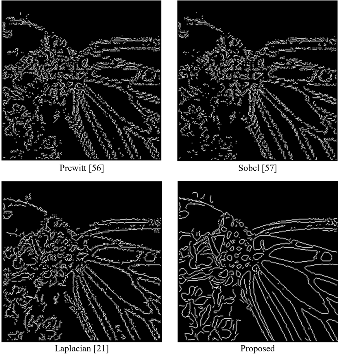
Figure 5.5: Comparative analysis of proposed approach with classical edge detection operators in FrFTD for Butterfly image (256×256)
