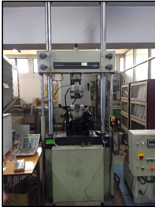
Figure 3.3 Tensile testing machine for testing at quasi-static strain rate (Courtesy: CSIR-NML, Jamshedpur).
