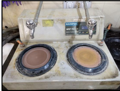
Figure 3.7 Polishing machine (Courtesy: CSIR-NML, Jamshedpur).
