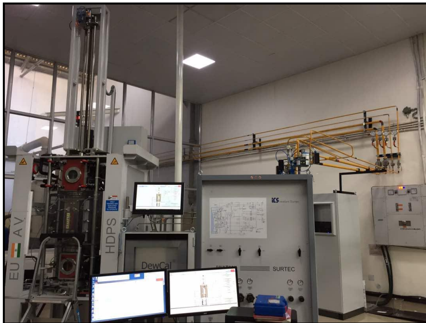
Figure 3.2 Hot dip process simulator used (Courtesy: CSIR-NML, Jamshedpur).
