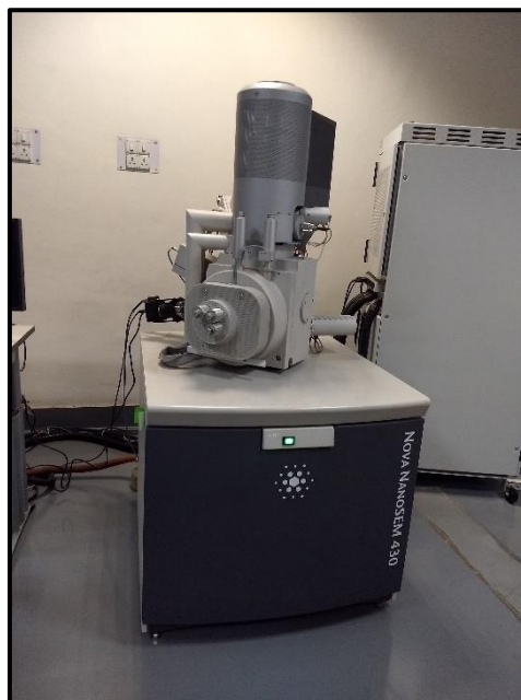
Figure 3.9 Field emission scanning electron microscope (Courtesy: CSIR-NML, Jamshedpur).
