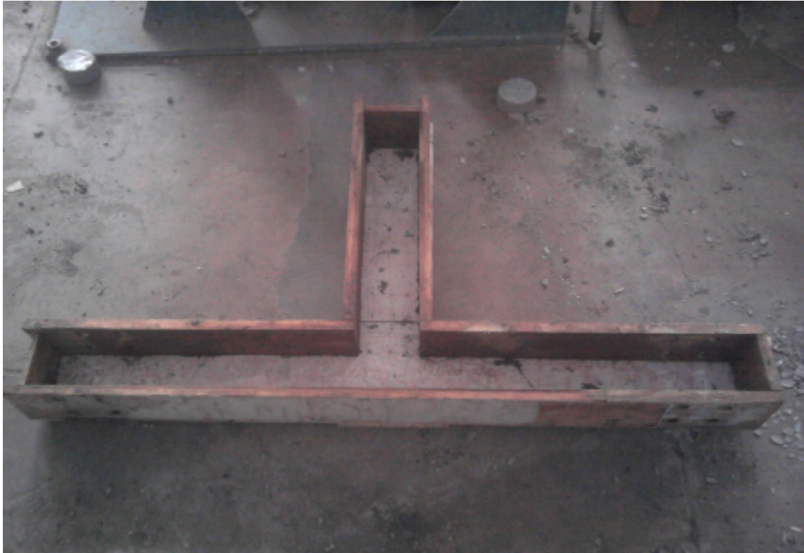
Plate 3.6: Wooden Mould Used For Casting of Beam Column Joint
