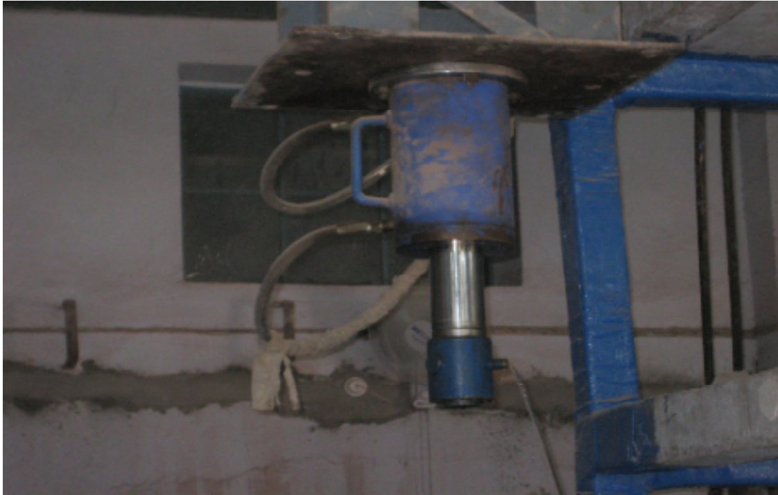
Plate 3.3: Testing Jack Showing Full Travel of the Jack
