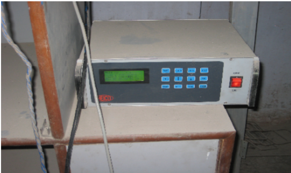
Plate 3.4 Data Acquisition System Connecting to Load Cell
