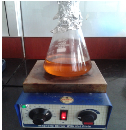
Transesterification set up of castor oil
