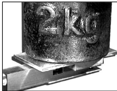
Figure-1.67. Linear stage with 10 mm stroke at Resolution of movement:atomic.2 nm resolution, burdened with 2 kg.
