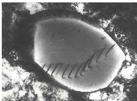
Figure-1.44. Transmission electron micrograph of dislocations in steel, which are faults in the structure of the crystal lattice at the atomic scale
