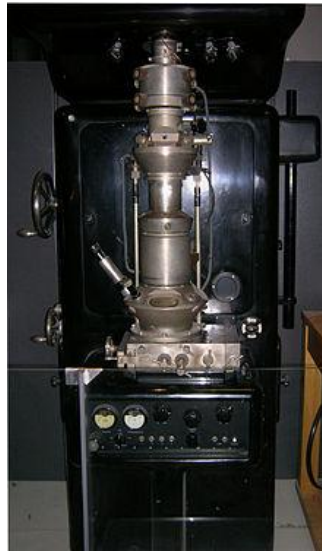
Figure-1.34. The first practical TEM, Originally installed at I. G Farben-Werke and now on display at the Deutsches Museum in Munich, Germany
