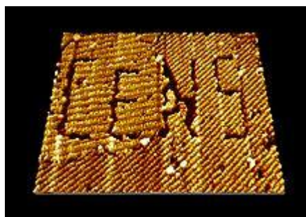
Figure-1.31. Nanomanipulation via STM of a self-assembled organic semiconductor monolayer (here: PTCDA molecules) on graphite, in which the logo of the Center for NanoScience (CeNS), LMU has been written.
