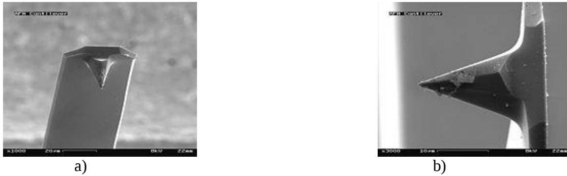
Figure-1.22. a) Electron micrograph of a used AFM cantilever image width ~100 micrometers. b) ~30 micrometers
