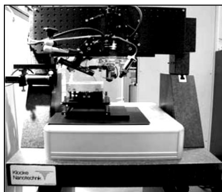
Figure-1.61. When a bigger high precision xy-stage is necessary there are two systems defined by the size of this stage: an xy-stage with 100x100 mm 2 stroke
