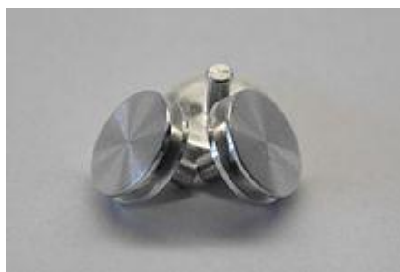
Figure-1.19. 13mm radius aluminium stubs (the base to support and prepare a sample on) for sample preparation and gold coating
