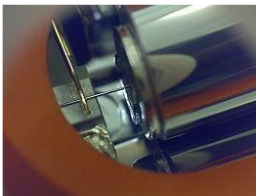
Figure-1.32. A close-up of a simple scanning tunnelling microscope head using a platinum-iridium tip.
