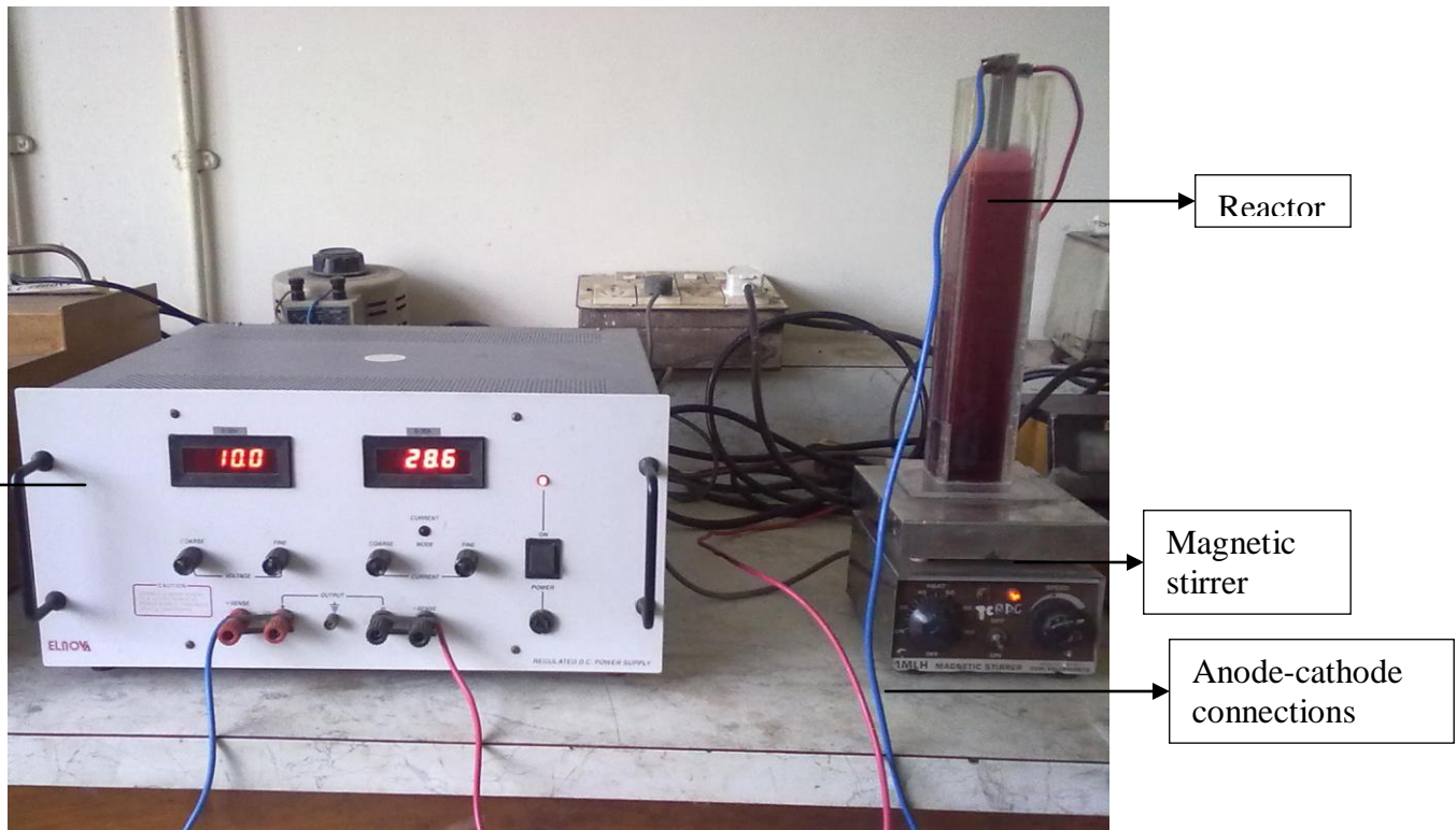
Fig.4.2.1. Experimental setup of electro flocculation
