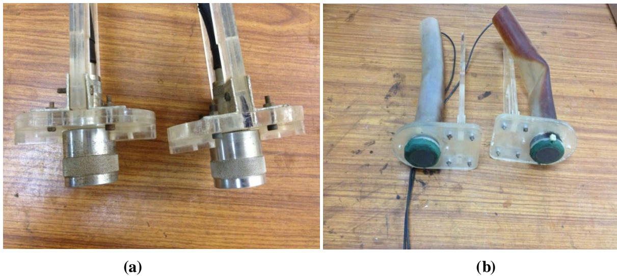
Figure 4.4: Immersion probes (a) 0.5 MHz (b) 1 MHz
