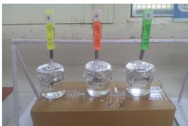
Figure 12. Substrates immersed in acidic solution of pH 3, 4 and 5
