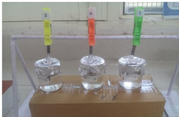
Figure12. Substrates immersed in acidic solution of pH 3, 4 and 5
