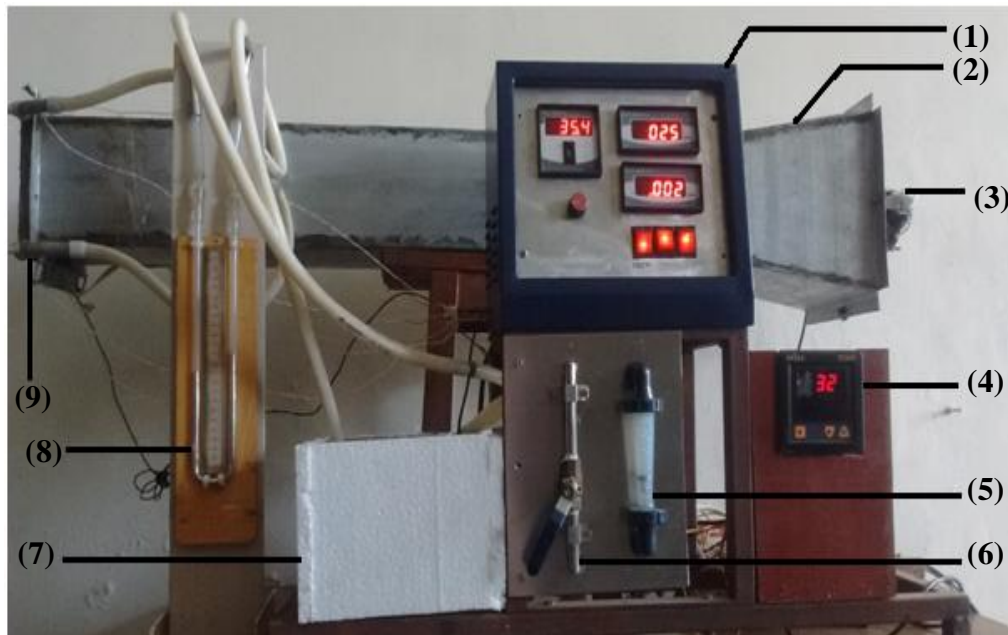
Figure 3.1: Experimental Equipment: (1) Display, (2) Air flow duct, (3) Forced draft fan, (4) PID controller, (5) Rotameter, (6) By pass valve, (7) Reservoir tank, (8) U tube manometer, (9) Heat exchanger.
