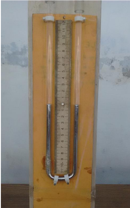
Figure 3.5: Mercury U Tube manometer
