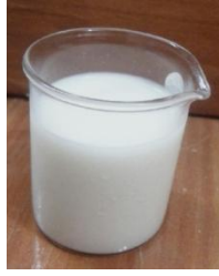
Figure.4.1: 0.1% volume concentration Al 2 O 3 /water and ethylene glycol (60:40) nanofluid
