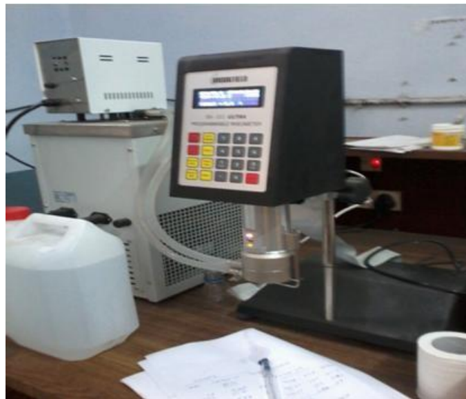
Figure 3.13: Brookfield DV-III Rheometer
