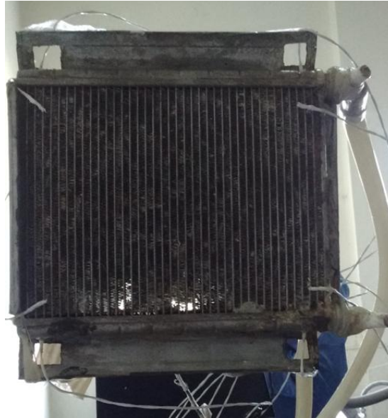
Figure 3.3: Heat exchanger with temperature sensors
