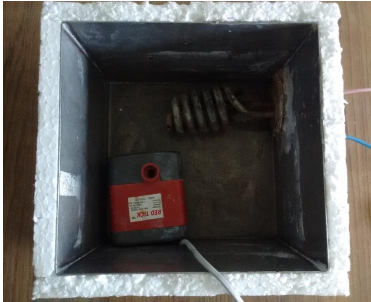
Figure 3.6: Reservoir tank with heating element and pump
