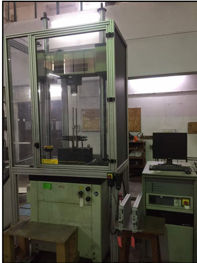
Figure 3.9: High speed servo-hydraulic Instron VHS 8800 test system for testing at high strain rates.
