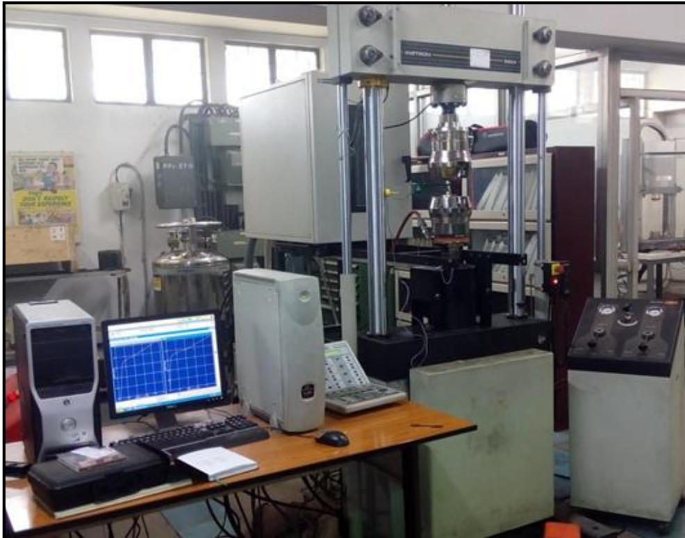
Figure 3.8: Tensile testing machine for testing at quasi-static strain rate.
