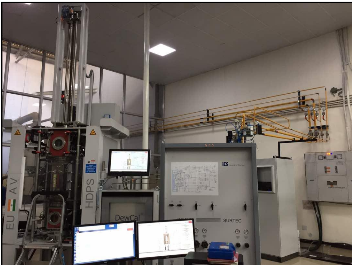
Figure 3.7: Hot dip process simulator used for annealing of samples.
