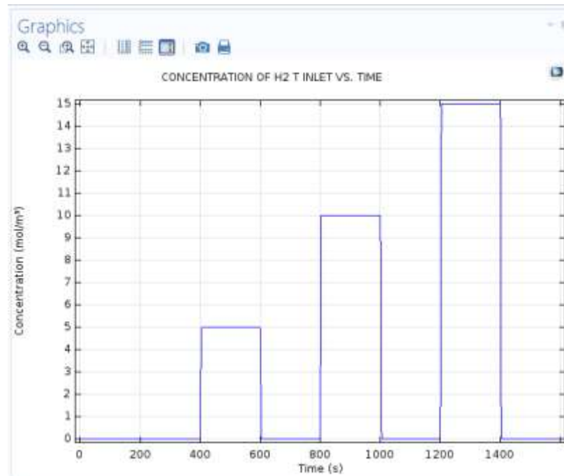
Fig 5.5 Input pulses of concentration given to the chamber
