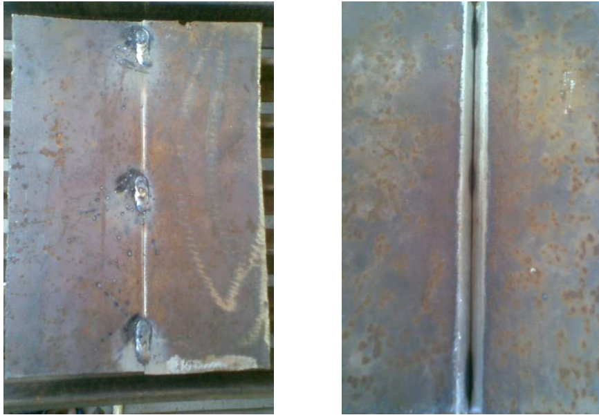
Fig 4.7: Tacking on back side of plates
