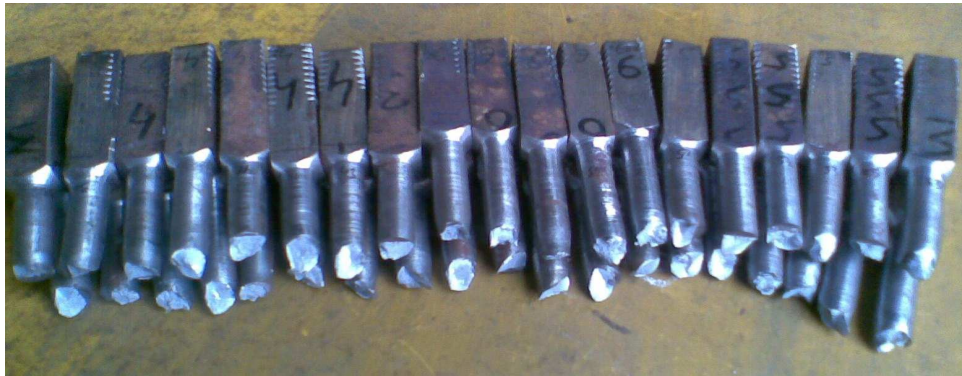
Fig 5.1: Specimen after tensile test
