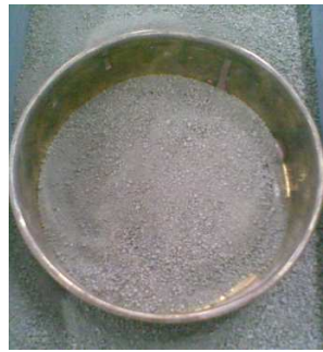
Fig 4.3: Test sieve (8 BS, 10 ASTM, 2 mm IS, 2057 microns)
