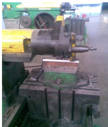
Fig 4.5: Making chamfer on corner of plate
