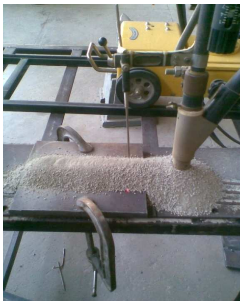
Fig 4.8: Submerged arc welding of plates
