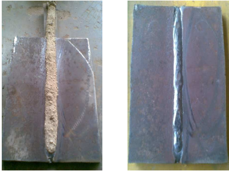
Fig 4.9: Joint of plates after welding
