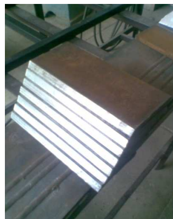
Fig 4.6: Chamfer on plate
