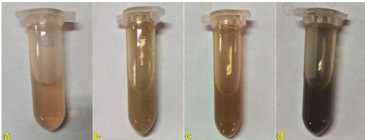
Figure 18: Change in colour due to reduction of silver nitrate by fruit extract at a) 1 hour b) 3 hours, c) 5 hours and d) 24 hours
