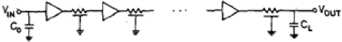
Figure 5.13: Optimum number of repeaters inserted to drive SWCNT bundle interconnects [15].
