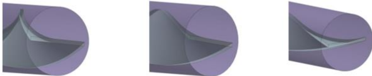
Figure 3.9: Geometry of different FLTT with different clearance ratios (3-D view)
