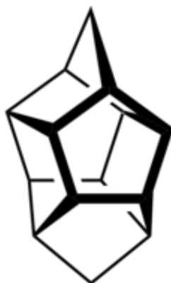
Figure 1.1 Pentasil unit of ZSM-5 zeolite
