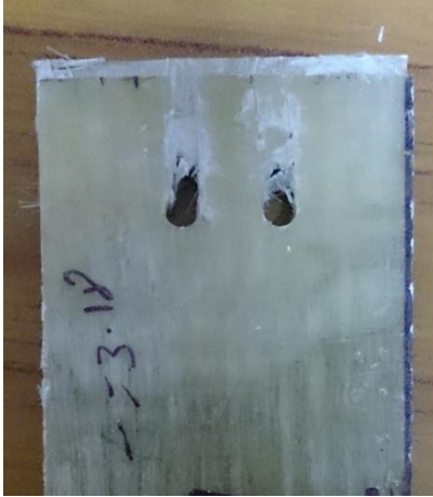
(e) E/D= 4 , K/D= 4 , P/D= 3 with bearing mode of failure
