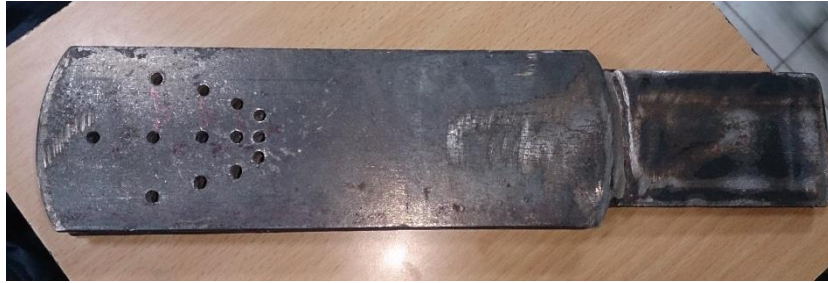
Figure 3.6: Fixture for double pin joint laminates
