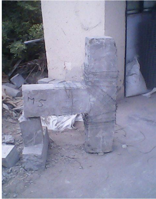
Figure 3.7 Specimen Retrofitted with Mesh Wire (Type Two Retrofitting).
