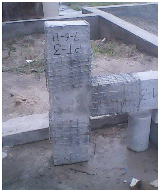
Figure 3.6 Specimen Retrofitted with Mesh Wire (Type One Retrofitting).
