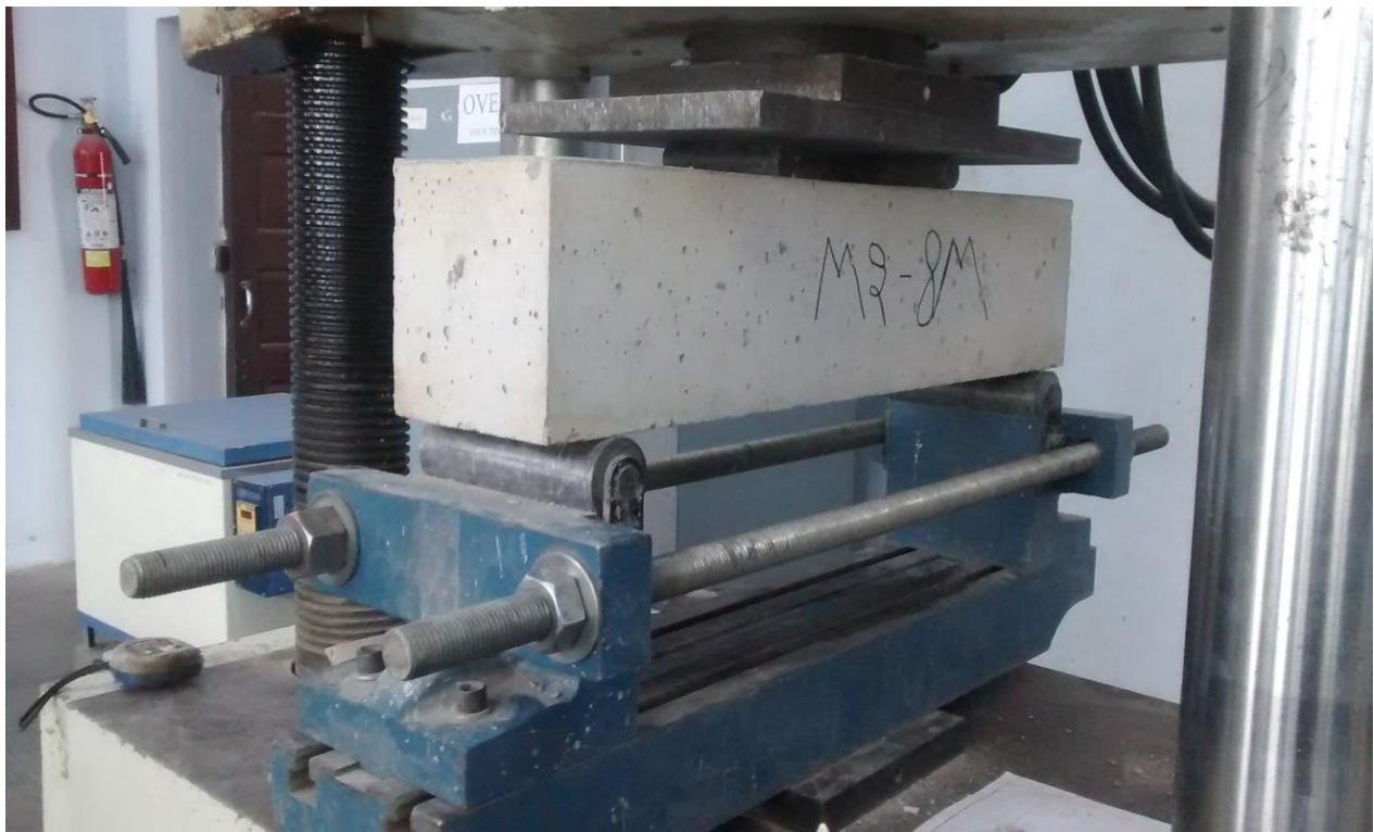
Fig. 3.8 Flexural Strength Test Setup
