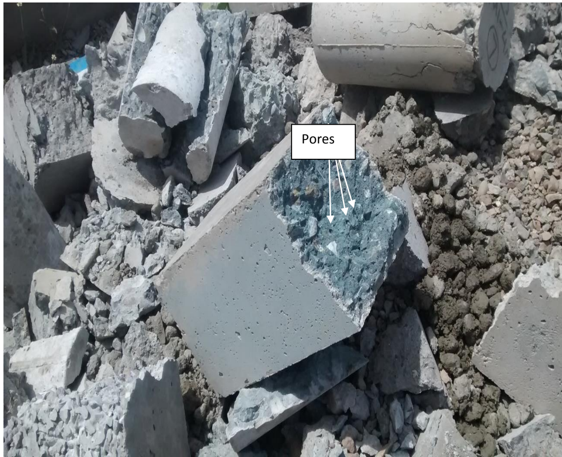
Fig. 1.2. Pores in the Cross Section of Broken Geopolymer Concrete Specimen
