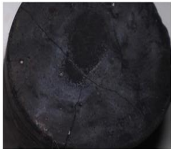
(d) A picture of cracks on the surface of an inorganic polymeric paste sample
