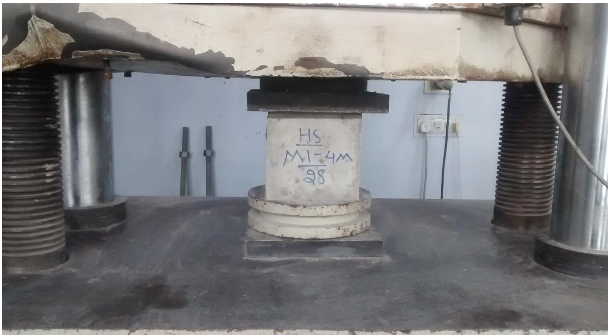
Fig. 3.7 Compressive Strength Test Setup
