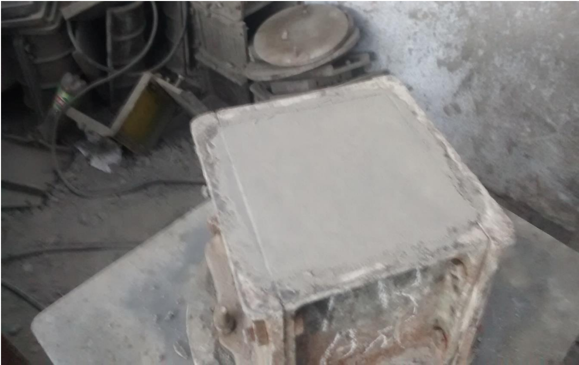
Fig 3.6. Finished Mould Containing Geopolymer Concrete
