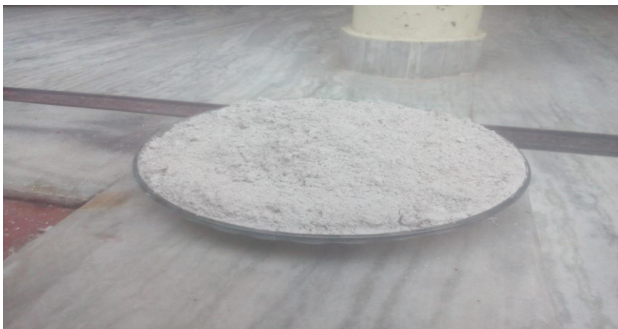
Fig. 3.3. Actual Photograph of GGBS
