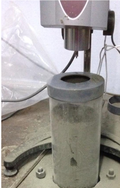
Figure 4.14: Channeling for cohesive Powder 3
