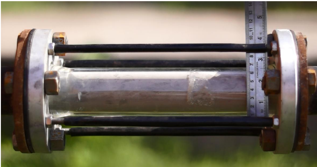
Figure 2.3 Dense phase (non suspension) flow
