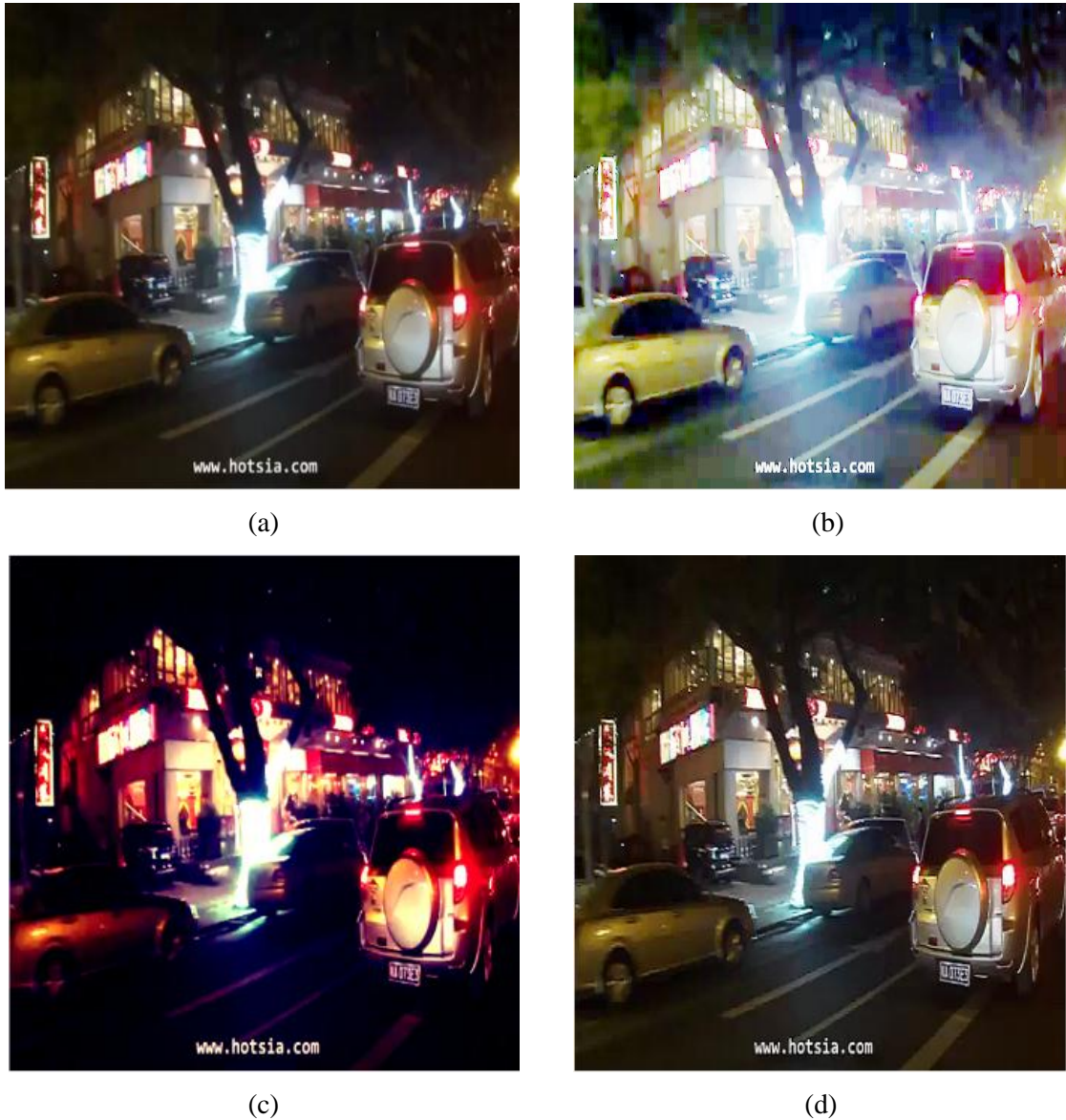
Figure 5.12: (a) Input video (1 st frame) (b) Enhanced 1 st frame by HE (c) Enhanced 1 st frame by LCA (d) Enhanced 1 st frame by proposed mask (improved G-L at 0.3 fractional differential order)
