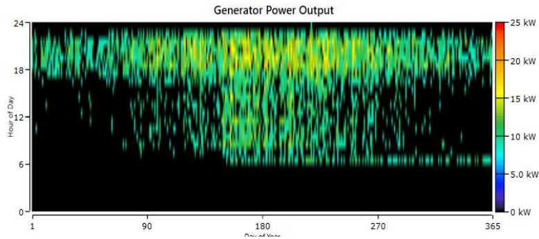
Fig. 4.14 Biomass Gasifier Production Yearly
