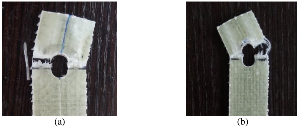
Fig. 3.27 Failure mode at w/d = 3 (a) Torque 0 Nm (b) Torque 5 Nm
