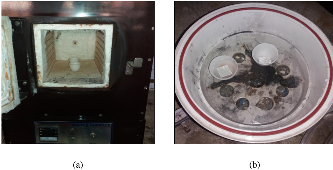
Fig. 3.5 (a) Muffle furnace (b) Tested sample in desiccator
