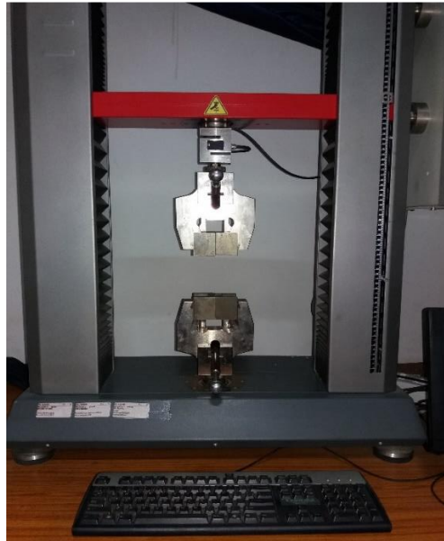
Fig. 3.6 Universal testing machine setup
