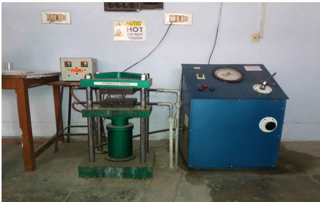
Fig. 3.3 Compression moulding machine
