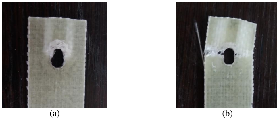
Fig. 3.28 Failure mode at w/d = 4 (a) Torque 0 Nm (b) Torque 5 Nm
