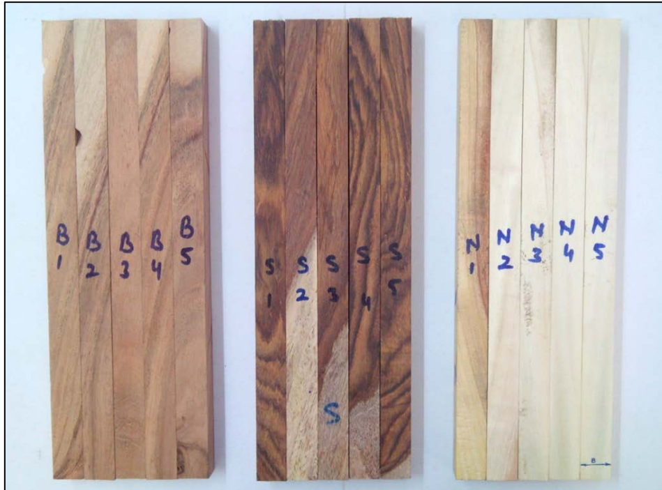
Figure 3.5: Specimens of Babool, Sheesham and Neem wood Species prepared for MOR and MOE test
