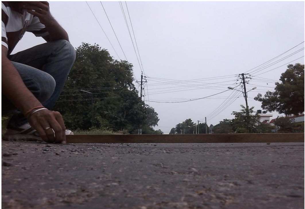
Plate 4.4: Rut Depth Measurement
