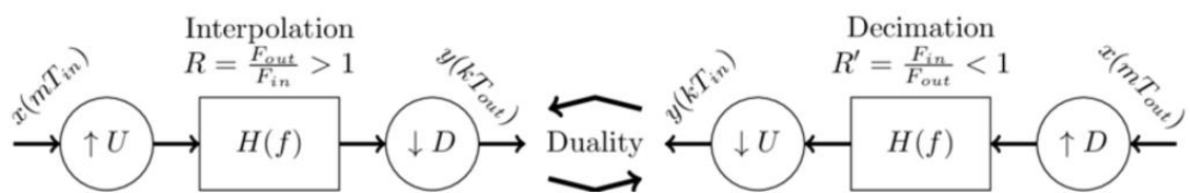
Figure 4.2 demonstrates the processes of interpolation and decimation in telecom. Interpolation shows how intermediate samples are inserted between original signal points to increase resolution, while decimation depicts the removal of samples to lower the sampling rate. [33].
