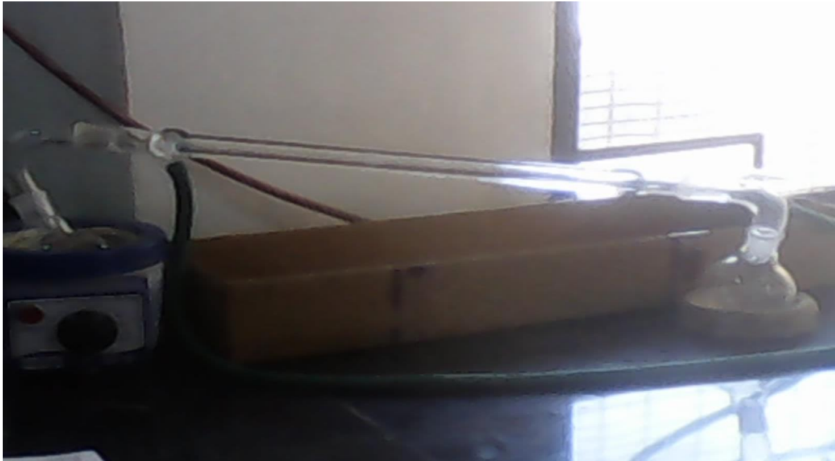
Figure 4.4 This above picture shows the Distillation column used in laboratory for pure Ethanol extraction from samples.
