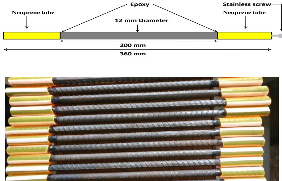
Fig. 5.3 Line diagram and actual prepared TMT steel bars
