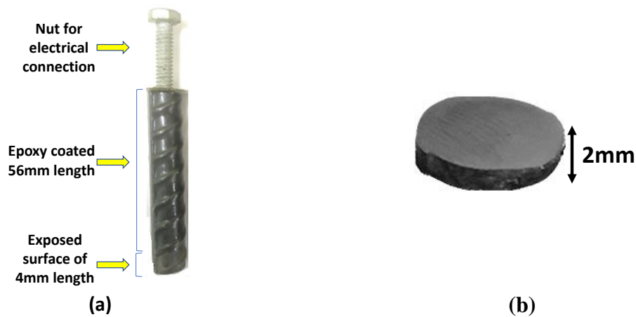
Fig. 3.2 Bare steel specimen prepared for (a) electrochemical tests and (b) surface analysis tests in synthetic pore solution
