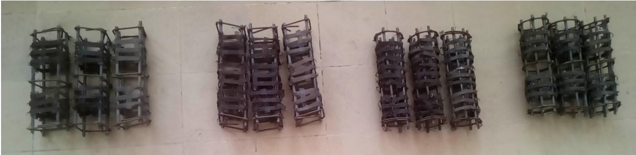
Fig.3.6: Geo-grid tied column specimens
