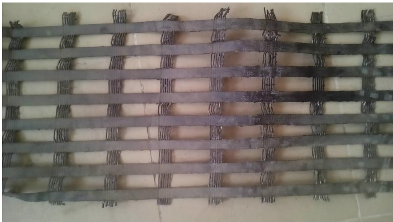
Fig.3.5: Geo-grid used in the study
