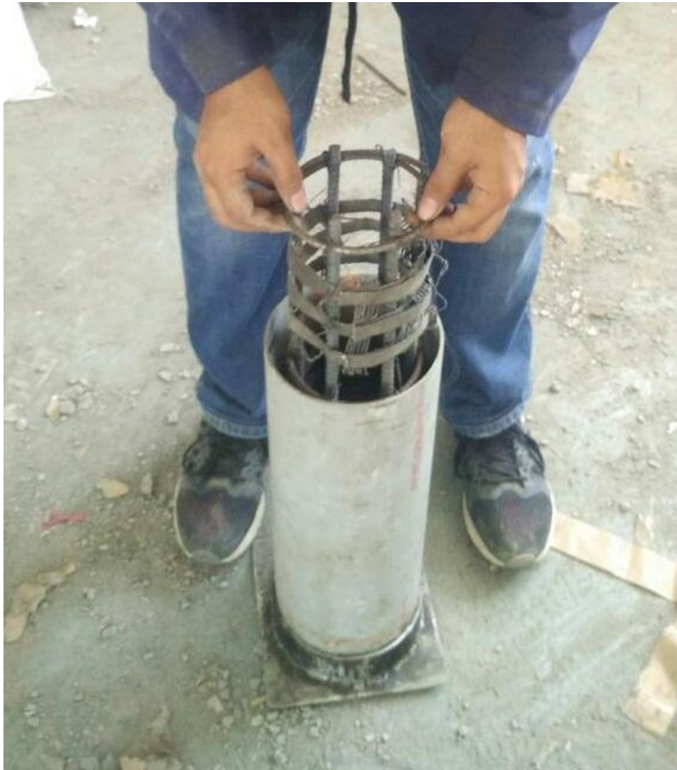
Fig.3.7: Preparation of circular column specimen
