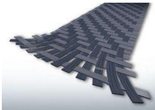
Fig.1.3 (d): Fiber Reinforced Polymer
