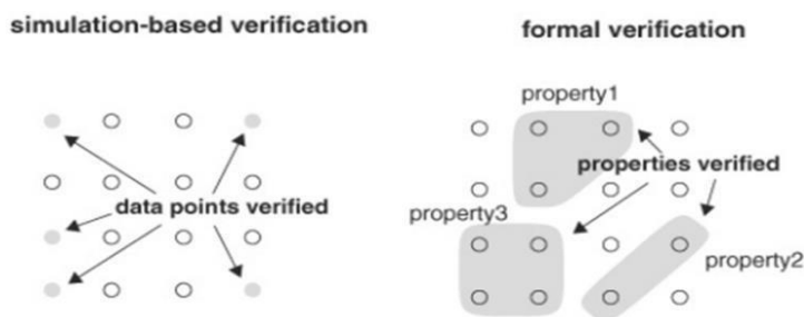
Figure. 4.6 An output perspective of simulation-based verification versus formal verification
