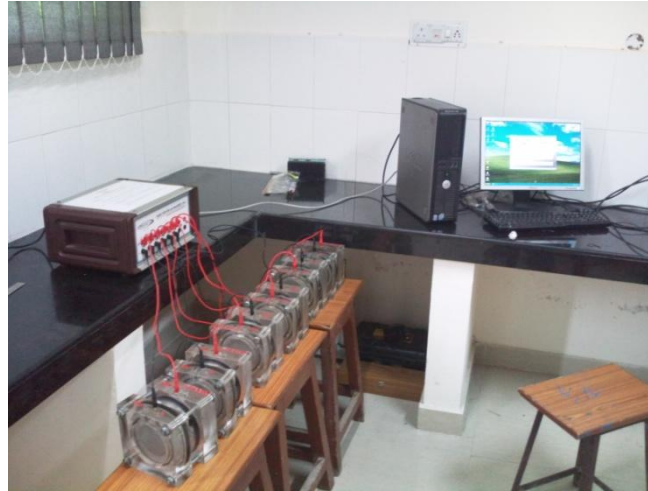
Fig. 3.8: Rapid Chloride Permeability Test Set Up
