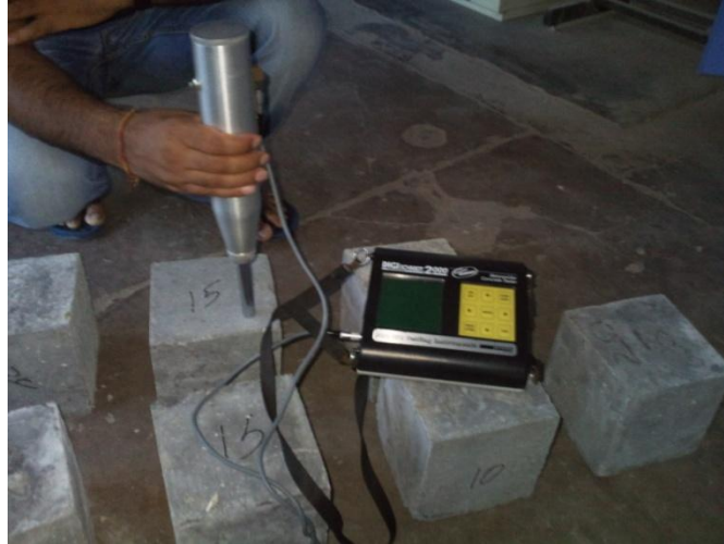
Fig. 3.10 Rebound Hammer Test
